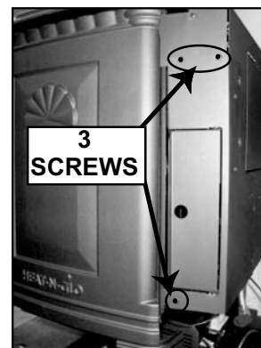
Figure 8.30 Remove valve access cover from back of appliance by removing the three screws indicated.
